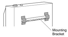
Figure 12 - Mounting Bracket Location
