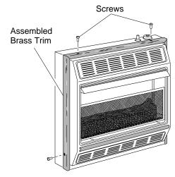
Figure 7 - Attaching Brass Trim to Heater
