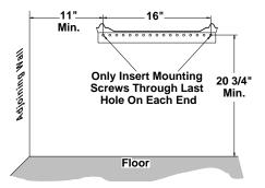
Figure 13 - Mounting Bracket Clearances
