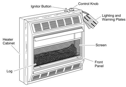
Figure 1 - Vent-Free Gas Log Propane/LP Gas Space Heater
