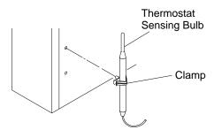
Figure 11 - Attaching Thermostat Sensing Bulb
