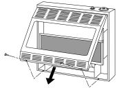
Figure 2 - Removing Front Panel of Heater
