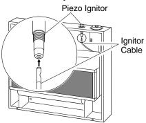
Figure 3 - Attaching Ignitor Cable to Piezo Ignitor Continued
