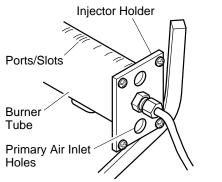
Figure 30 - Injector Holder On Outlet Burner Tube
