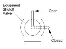
Figure 22 - Equipment Shutoff Valve
