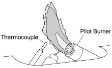
Figure 27 - Incorrect Pilot Flame Pattern
