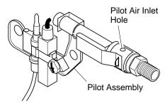
Figure 31 - Pilot Inlet Air Hole
