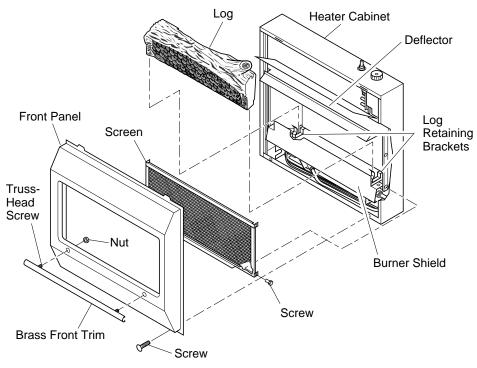
Figure 4 - Assembling Heater
