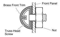
Figure 5 - Attaching Brass Front Trim to Front Panel
