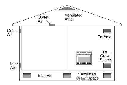
Figure 9 - Ventilation Air from Outdoors
