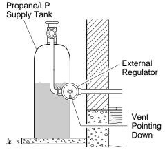
Figure 20 - External Regulator with Vent Pointing Down
