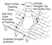
Figure 15 - Flashing Installation
