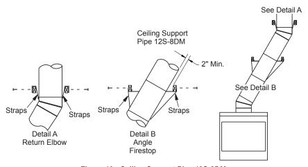
Figure 10 - Ceiling Support Pipe 12S-8DM
