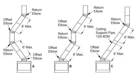
Figure 9 - Typical Offset Installation
