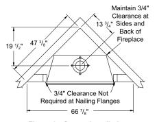
Figure 2 - Corner Installation
