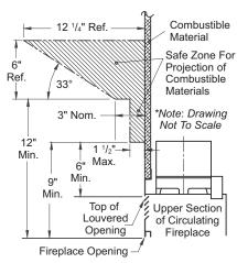
Figure 4 - Mantel Clearances to Combustible Material
