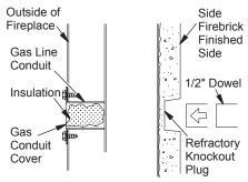
Figure 21 - Gas Line Knockout
