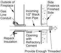
Provide Enough Threaded End for Fitting Connection
