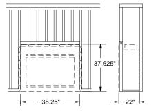
Figure 1 - Framing Dimensions
