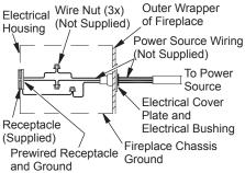
Figure 6 - Fan Switch-Electrical Bushing
