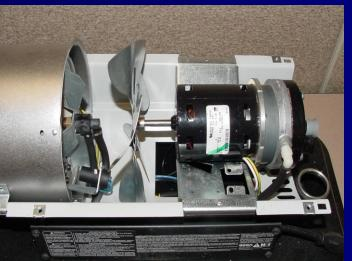
Connect the yellow wires to the open terminals on the control board.
