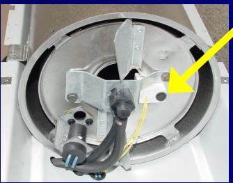
Remove the screws holding the side-panel and control board in place. Disconnect the yellow wires.
