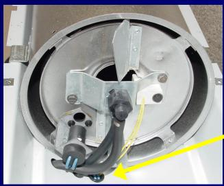
Tighten down the screw and route the wires down into the cavity below.
