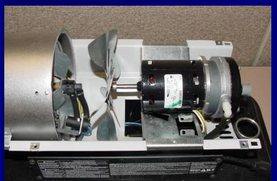
You can now see the combustion chamber and fan motor assembly.
